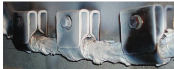
Phoenix clips have been fire tested in accordance with BS 5839-1: 2017.
