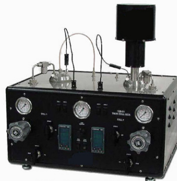
A Single SGSM Unit on a 5,000 PSI Twin Cell UCA
