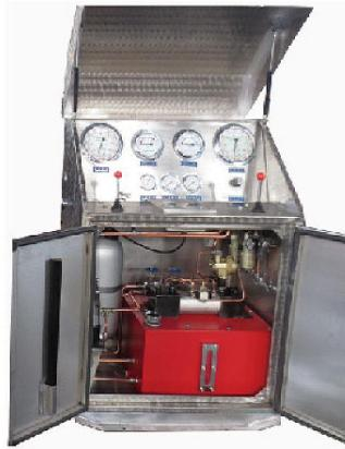
Control panel is the control device for hydraulic choke manifold. It can remote control the opening and closing of the hydraulic choke valve and show the pressure of standpipe and casing pressure, and the switching position of hydraulic choke valve. It can also show the strokes and frequency of the three mud pumps if equipped with pump stroke counter, which is an necessary equipment to control well kick, blowout and pressure balance.
