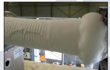
Hose filled with LIN during 9 weeks.
