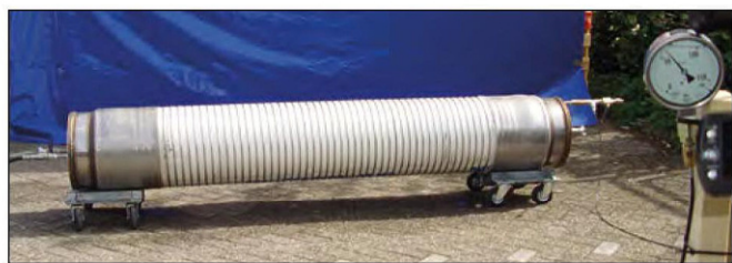
Ambient burst test on prototype Multi-LNG White 16"
