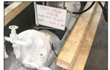
8" Multi-LNG White STS crushed with external loads up to 160 kN. Internal hose pressure of 6 bar. Done both ambient and cryogenic without any leakage.
