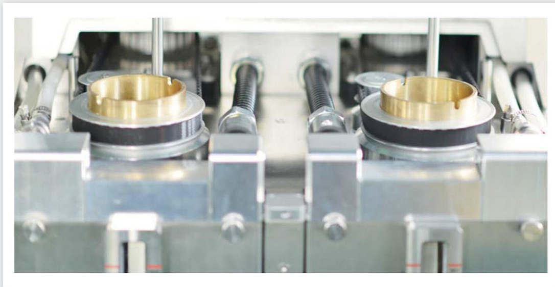
Easy-to-disassemble Water Baths & Cooling Water Pipes and Power Supply Cables with Quick Couplings
